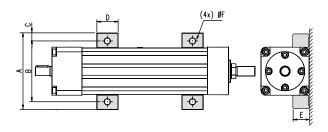
The movable mounting feet clamp accessory is only available for T60 units. This option can be mounted on the unit from the factory if stated in the ordering key at order, in which case you get four clamps, or they can be ordered as separate pieces using the part number. Normally you would need four clamps per unit. The clamps fit into the T-slot running along each side of the unit.
